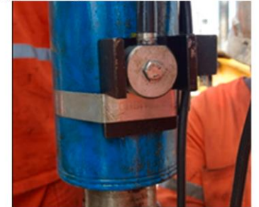
(b) fastening detail of the accelerometers
